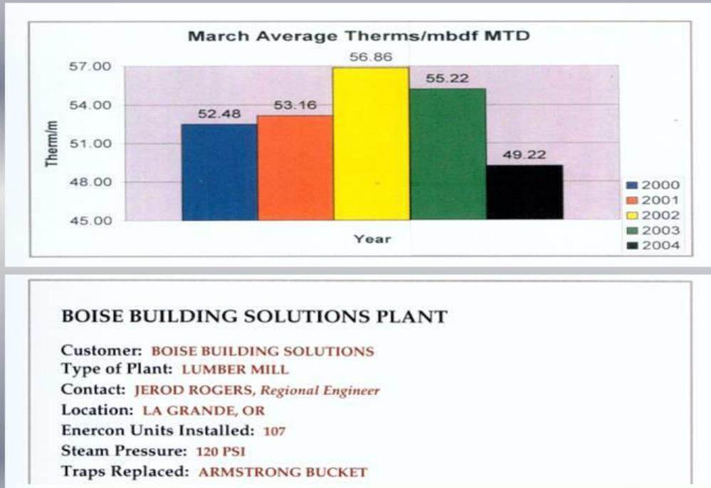
*This is an example of return side improvement. The black bar is after the installation of the EVCR Units. This is a natural gas system showing a significant reduction in fuel consumption.*
