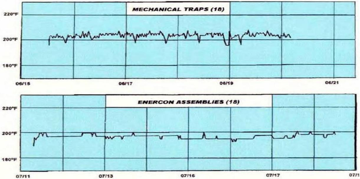
**TEMPERATURE PROFILE TEST COMPARING ENERCON WITH MECHANICAL TRAPS**
