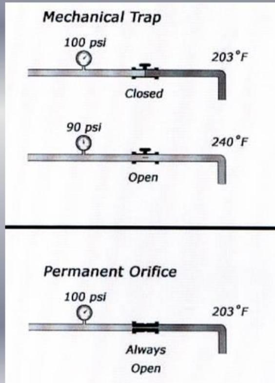
*A simple experiment can be performed by any customer using steam. If you put a pressure gage before a mechanical trap, the pressure drops every time the trap opens. At the same time, the return temperature will rise significantly above accepted heat loss levels. The orifice will discharge the same condensate with no movement on the pressure gage and will permanently maintain accepted heat loss levels.*
