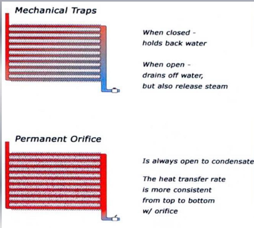
*This is a comparison to show why the EVCR Units accomplished what they do in coil related operations. The mechanical traps are closed for the majority of the time while the coil is still transferring heat. This reduces the energy to pound mass and the total heat transfer capability of the coil. It also, creates a severe temperature variance from the inlet to the outlet of the coil which causes uneven drying. With the EVCR Units, these problems are dramatically reduced.*
